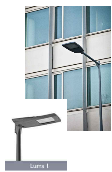
Philips Luma 1A R5 DS-CW 1 Spigot mounted 6m x 76mmØ tubular column Powder coated to RAL9006
